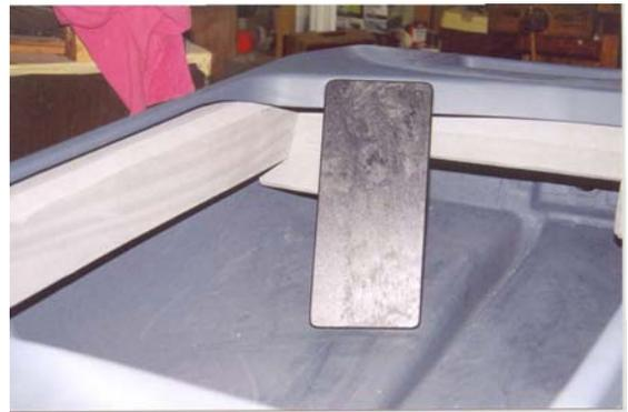
**The entire floatation system of the boat has been redesigned with rail mounted, foam filled ABS Floatation Tanks. There is an ABS piece designed to fit the stern to encapsulate the urethane floatation foam along with the poured foam in the bow. This gives us even more floatation than is required and provides you with an added margin of safety should it ever be needed. During assembly, you may also add/have added an optional S/S tow/anchor eye.**
