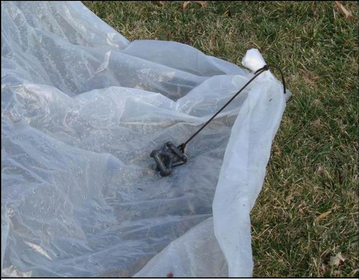
Here's the clamps we use for attaching to the outer edge of the curtain....any hardware store i.e. pick them up from Northern Cashway Lumber when you're getting the visqueen. ;) Most building supply houses will stock visqueen & clamps.
