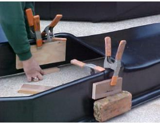
The top and bottoms are now pre-assembled. It's time to gunk up the top flange of the bottom unit with a good heavy bead of gunk (1/4" to 3/8" bead).
