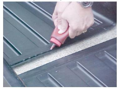
Join the two pieces as shown....gently & accurately placing the pieces together for proper alignment. Clamp them at the upper edge & sides. Place some bricks or heavy objects onto the bottom seam to be sure you are getting a good solid,full contact joint. Allow at least 2 hours drying time before removing clamps and continuing with assembly.
