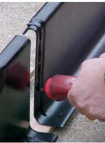
Once you have the pieces "gunked", assemble and clamp the top edge and sides. You can use pieces of plywood to spread out the clamping pressure and bricks to hold down the lower flange. Allow at least 2 hours drying time before removing clamps and continuing with assembly (overnight if using a slower adhesive-test first to assure yourself of cure time).
