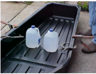
It's time to work on the deck. Place the deck on a flat surface or you may place it on top of the bottom unit that you've already assembled. If placing on the bottom unit, be sure to put something under the top joint when gluing to keep from bonding to the bottom at this time (masking tape works well). Squeeze a generous bead of gunk (1/4" to 3/8" bead) onto the depressed flange of the top unit as you did for the bottom.
