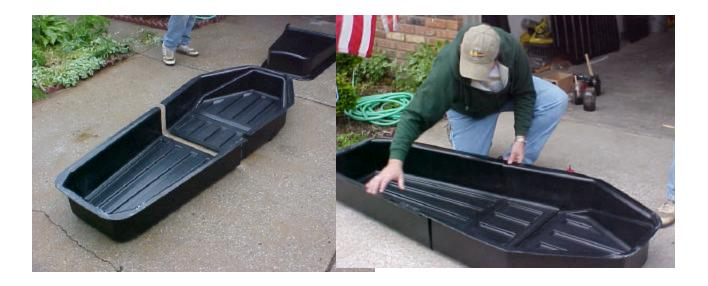
Squeeze a 1/4" to 3/8" bead of gunk onto the "depressed" flange of the front piece so you'll get a good joint and full fill-in for waterproofing. If you are using ABS adhesive, coat both surfaces prior to assembly.
